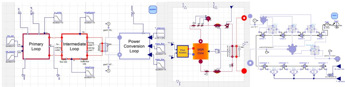
Figure 1: Plant simulator developed in the SAMOFAR project, to be adopted in the proposed analyses.
