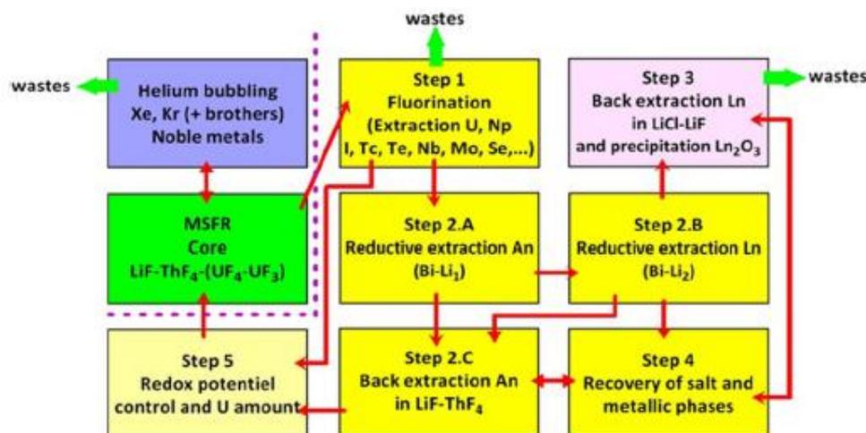
Figure 1: Schematic overview of the fuel processing stages in the fuel treatment unit [1].
