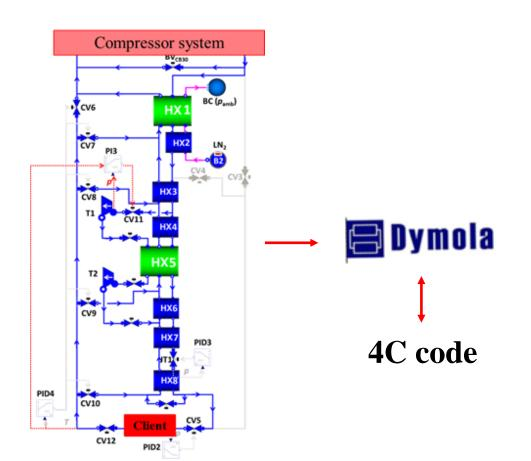
• <u>Problem</u>: the He refrigerator and the SC magnets are tightly coupled, especially during cooldown operation
